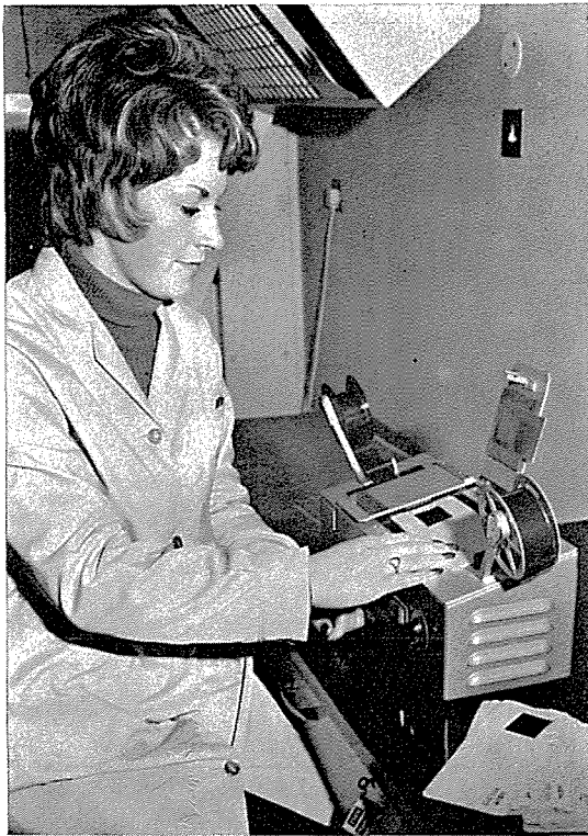
Mrs. Margaret Edwards, above , producing duplicate working aperture cards from an original 35 m.m. silver image film, which is kept as the master copy. Mr. Adrian Chesworth, below, left , extracting information with the aid of a viewer, while Mr. Howard Pearson inserts an aperture card into an electrostatic printer which in about ten seconds, produces a full-scale reproduction on paper.
